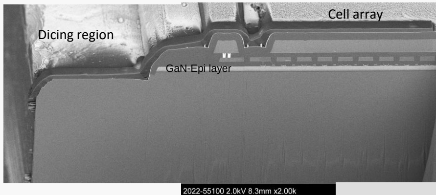
Die edge cross section SEM image
