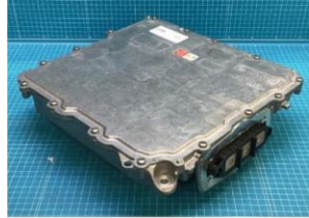
Rear Inverter Overview
